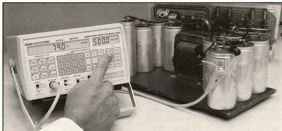
Figure 3: Capacitor banks are used to obtain a high CV rating.
