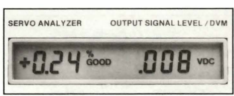
Fig. 1: The Servo Analyzer readout displays the test result as a percent-of-error reading and "Good/Bad" indication.
