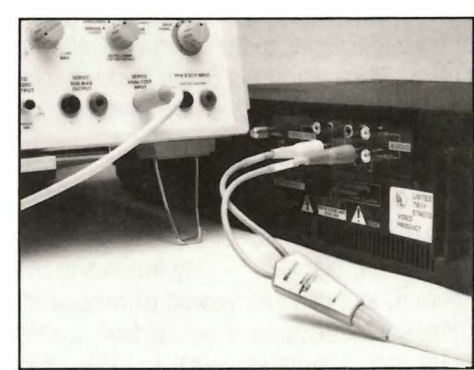
Fig. 2: The Servo Performance Test Lead easily connects to the VCRs video and audio output jacks for a quick check of the servos.
