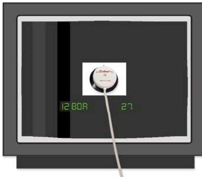
**Fig. 6: Select the 90 IRE Window pattern and adjust the CRT drive/gain controls for proper balance.**
