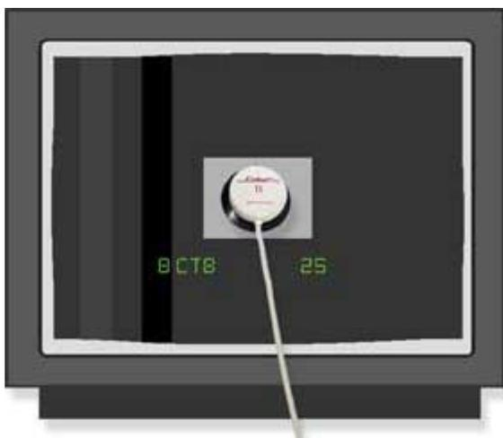
**Fig. 3: Select the 30 IRE Window pattern and attach the color pod over the center of the window. Adjust the CRT bias/cutoff controls for proper balance.**
