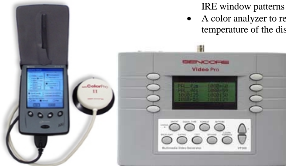
Fig. 1: Use the CP291 to quickly and accurately measure color temperature and use the VP300 to provide adjustable IRE level Window patterns.
