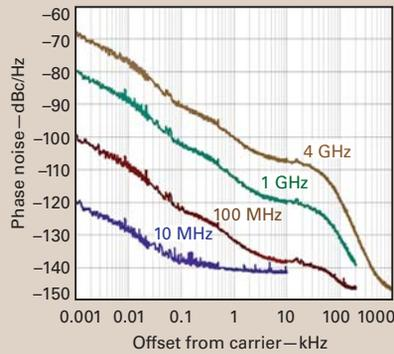
**2. The SG384 signal generator employs a unique frequency-synthesis technique to achieve low phase noise close to the carrier while also maintaining fine tuning resolution.**
