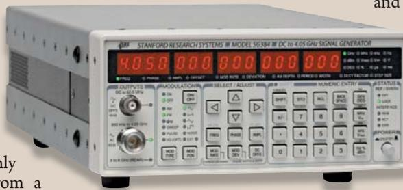
**1. The SG384 is a compact analog signal generator with frequency range of DC to 4.05 GHz (and to 8.10 GHz with a frequency-doubler option) and excellent spectral purity.**
