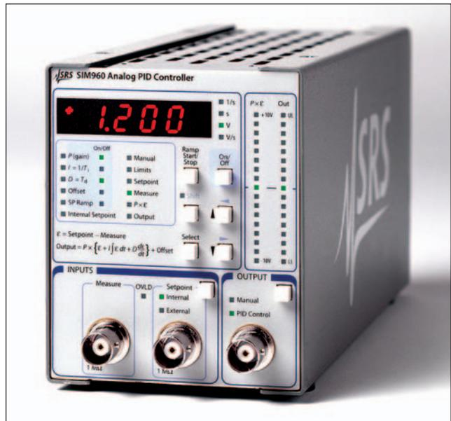
*The SIM960 Analog PID Controller is a broad-bandwidth, all-analog controller with front-panel adjustable gains and built-in anti-windup and bumpless transfer features.*
