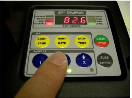
Students can 'flag' critical points in the melting process with the blue buttons on the keypad. Above are views through the lens showing a sample of vanillin during pre-heat, at the meniscus point, and at the clear point. After the melt is over (cooling LED is lit), the data are retrived by pushing the buttons again.
