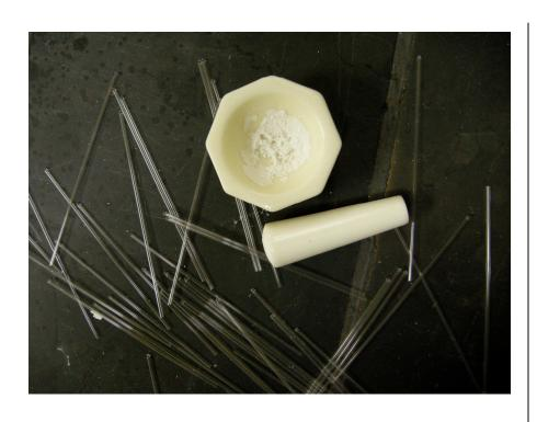
When students tap sample into capillaries, lots of capillaries end up on the floor, lots of capillaries are broken, wasted
