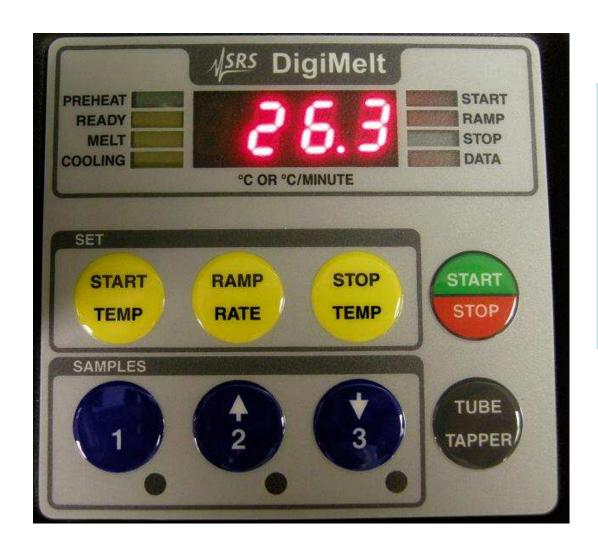
The keypad makes setting up a melt program very easy. The students push the yellow 'START TEMP' and then use the blue buttons with arrow keys to set the starting temperature. The students do the same for the 'RAMP RATE' and 'STOP TEMP' keys. Once the parameters are entered, they push the 'START/STOP' button and the microprocessor takes care of heating the block.
