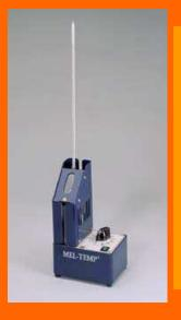
Note that the accuracy of the thermometer isn't really the accuracy of the MelTemp. The device must be calibrated against melting point standards to give a slope and offset correction to the thermometer reading. DigiMelt
