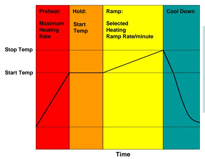
The student uses the keypad to enter a start, stop, and a rate. The microprocessor quickly heats the oven to the desired start temperature (typical time to 100 C is 2.5 minutes). After stabilizing at the start temperature, the microprocessor begins the melting ramp at the specified rate. Once the stop temperature is reached, the oven goes into cool down.
