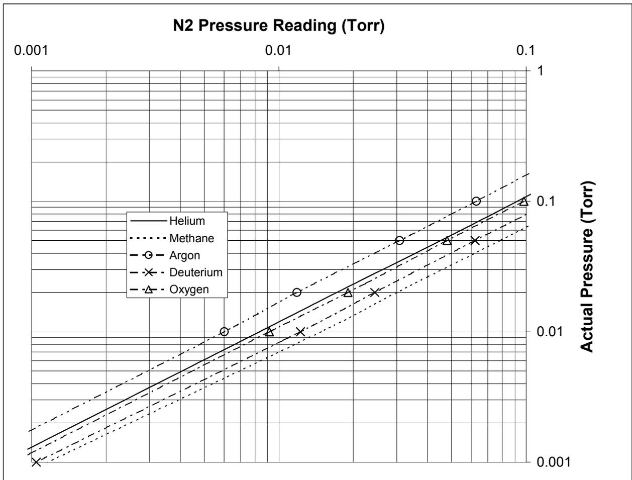
Figure I-1. PG105 Gauge Indicated Pressure (N<sub>2</sub> equivalent) vs. Actual Pressure Curve: 10<sup>-3</sup> to 10<sup>-1</sup> Torr.
