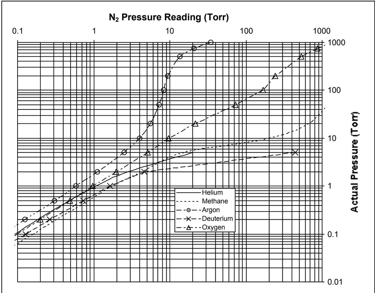
Figure I-2. PG105 Gauge Indicated Pressure (N<sub>2</sub> equivalent) vs. Actual Pressure Curve: 10<sup>-1</sup> to 1000 Torr. Use only when gauge axis is horizontal.
