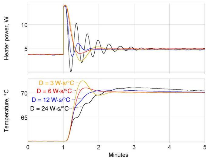
With the right amount of derivative feedback, we can increase  $P$  and  $I$  to levels that would otherwise cause oscillations, and thereby obtain faster, more responsive feedback control.
