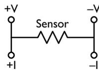
Four-wire sensors usually have two wires of one color attached to one side of the RTD, and two of a second color attached to the other side. In this case, the RTD should be wired to the PTC10 in one of the following two ways (assuming the leads are white and black):
