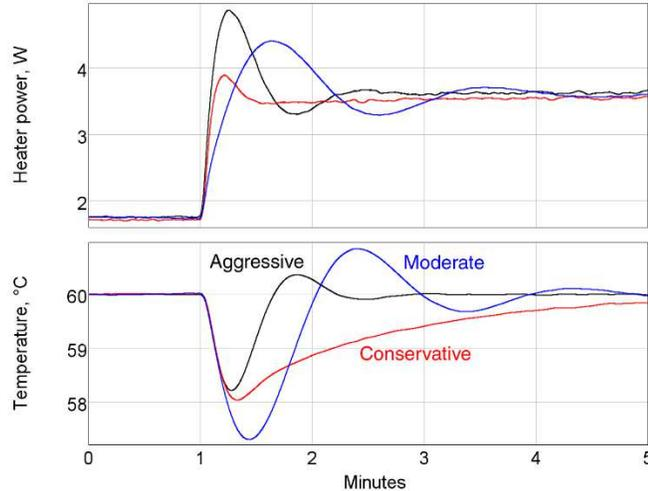
The actual behavior of your system might vary significantly from the behavior shown in these figures. In any event, the feedback gains determined by the automatic tuning algorithms should generally be regarded as only a starting point. In critical applications, the gains normally need to be manually adjusted to achieve good feedback performance.
