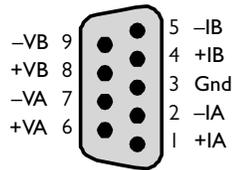
Sensor In 1, for example, should be connected to pins +IA, -IA, +VA, and -VA as described below. Cable shields should be connected to pin 3, which is chassis ground.
