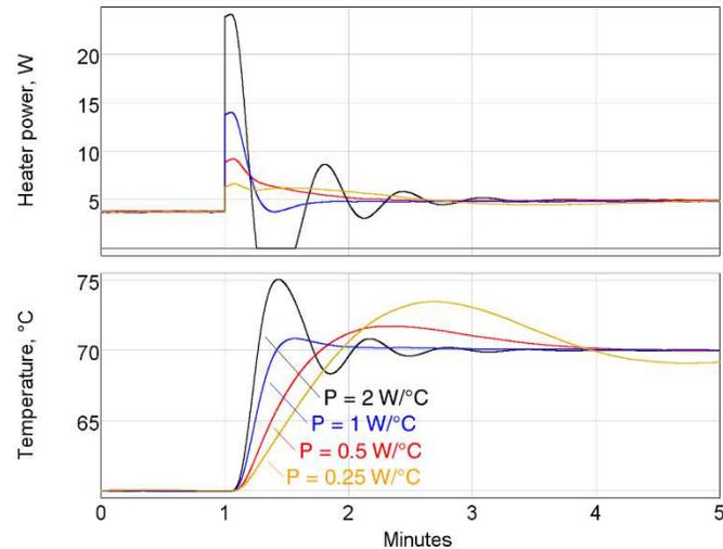
Interestingly, decreasing the proportional gain to 0.5 or 0.25 W/°C also results in more overshoot and can even cause oscillations, despite the fact that the heater response is smaller and the temperature rise slower. By reducing the proportional feedback response, we've forced the integral feedback to take more responsibility for raising the heater power — and as the next figure illustrates, the integral feedback has a greater tendency to overshoot and oscillate.
