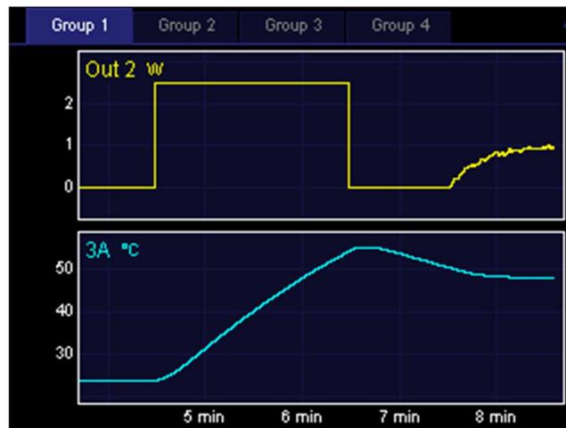
Heater power (top) and sensor temperature (bottom) during step response autotuning. Step Y is 2.5 W, Lag is 45 s, feedback is initially off, and the system starts at room temperature. After the step response is complete, the feedback turns on and the temperature drops before stabilizing at the  $50^{\circ}\text{C}$  setpoint.
