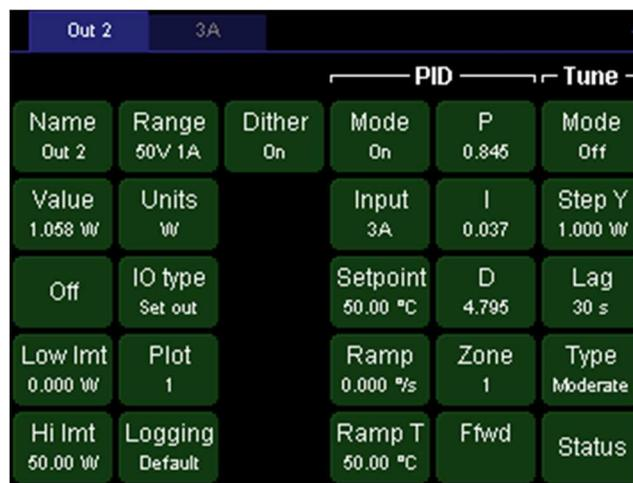
The "Channel" screen includes controls for all settings that affect individual data channels. Sensor calibration, PID feedback parameters, and alarms are all set up through this screen. Note that the layout of the screen varies depending on which channel is selected; for example, only output channels have PID controls, while only input channels have alarm controls.
