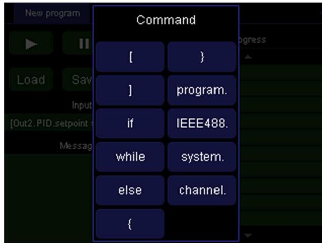
Any button with a name ending in a dot brings up a sub-menu when pressed. For example, the commands to change the feedback setpoint or alarm limits for a channel are accessed by first touching the “channel” button.
