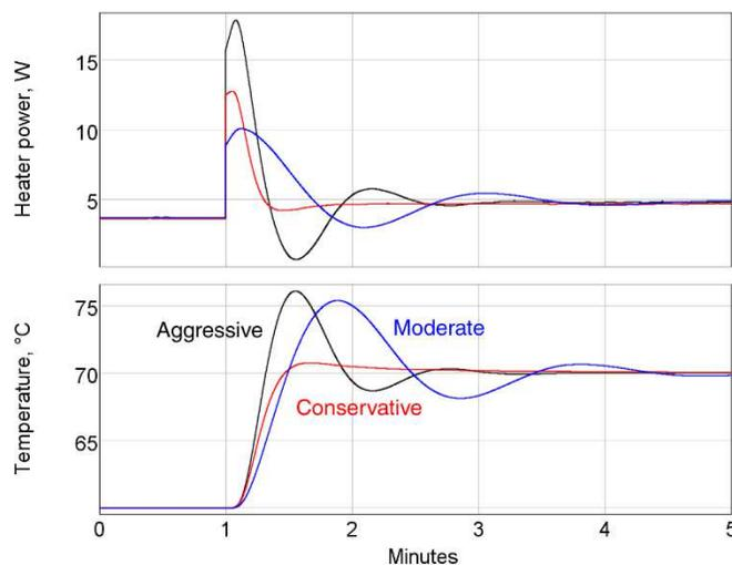
However, the results are much different if we look at how the system responds to a thermal disturbance. The next figure shows how well the system recovers when we start blowing air over the heater with a fan. The setpoint is a constant 60°C. In this case, aggressive tuning produces the best response.
