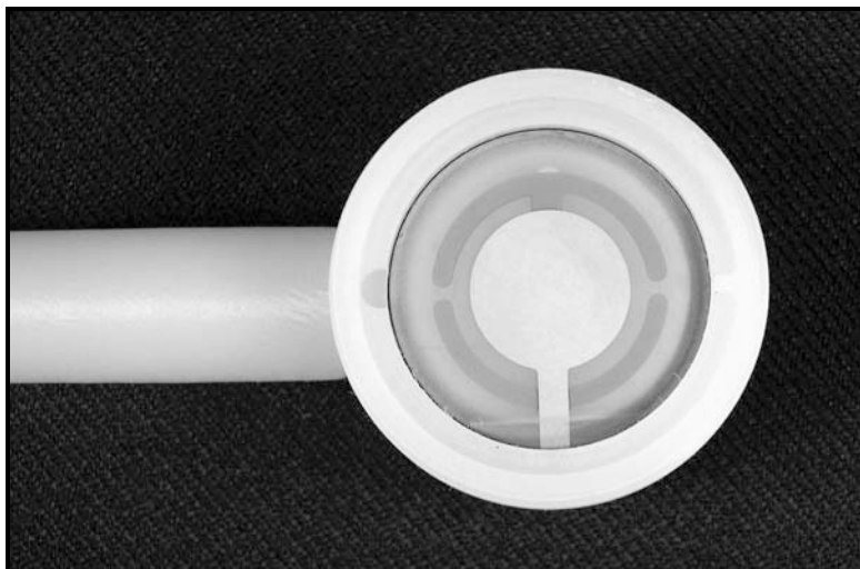
Figure 9. Crystal in place with correct electrode orientation.
