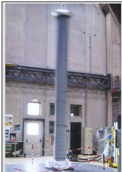
Seismic Qualification Test According IEC 60068 and U-SD1, Rev. 5; 1.0g with horizontal acceleration of 1g at first own frequency
