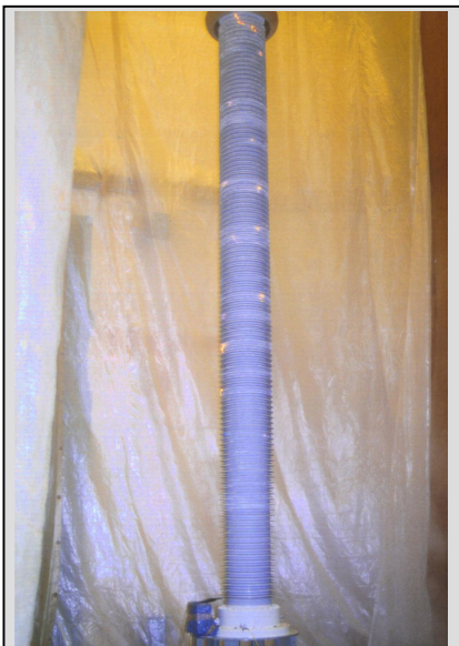
Artificial Pollution Test According IEC61245 Solid layer method with SDD of 0.04 mg/cm 2 at – 525kV DC
