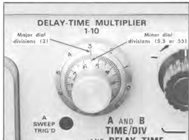
Fig. 2-17. DELAY-TIME MULTIPLIER dial. Reading shown: 3.55.
