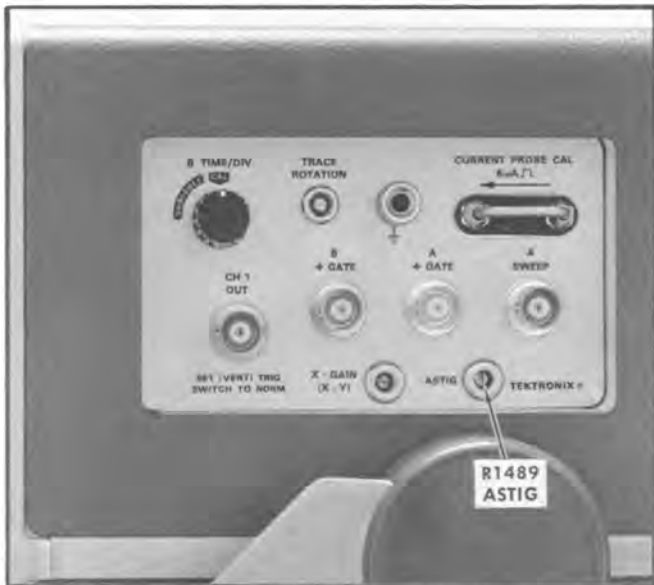
Fig. 6-12. Location of ASTIG adjustment (side panel).
