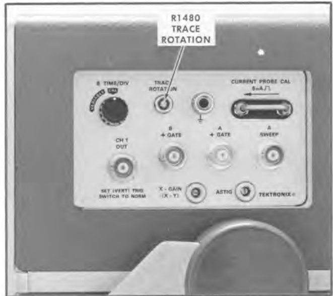
Fig. 6-10. Location of TRACE ROTATION adjustment (side panel).
