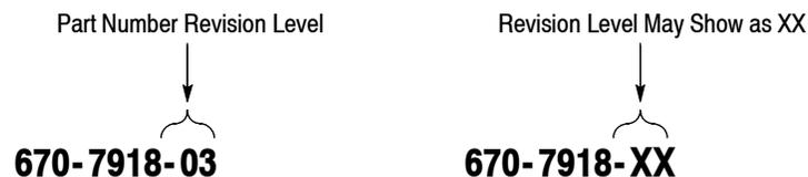
When you order parts, Tektronix will provide you with the most current part for your product type, serial number, and modification (if applicable). At the time of your order, Tektronix will determine the part number revision level needed for your product, based on the information you provide.
