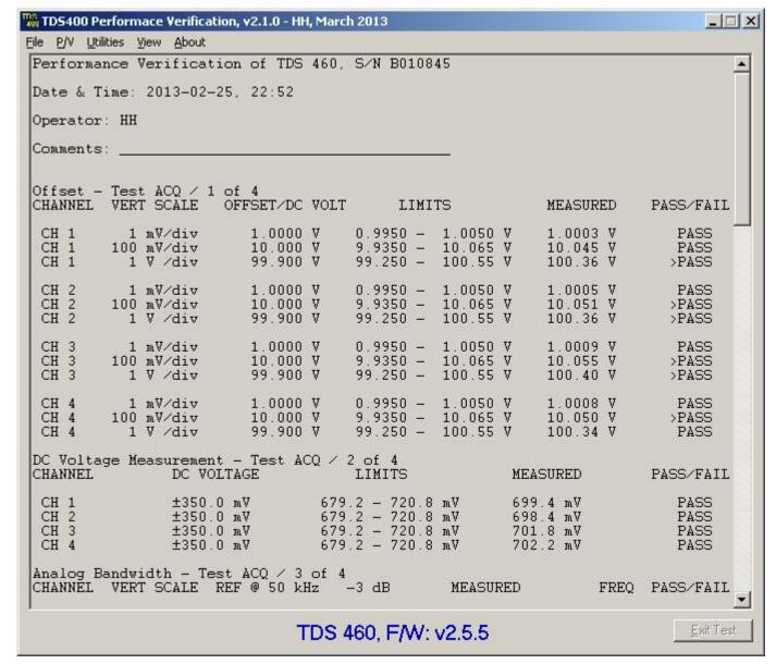
The > before PASS occurs when the result is more than 70% of the given limit and off course should the result be outside the limit FAIL will show.
