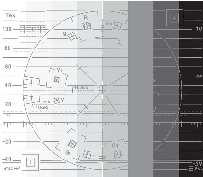
Figure 2-15. Picture mode display of color bar signal.
