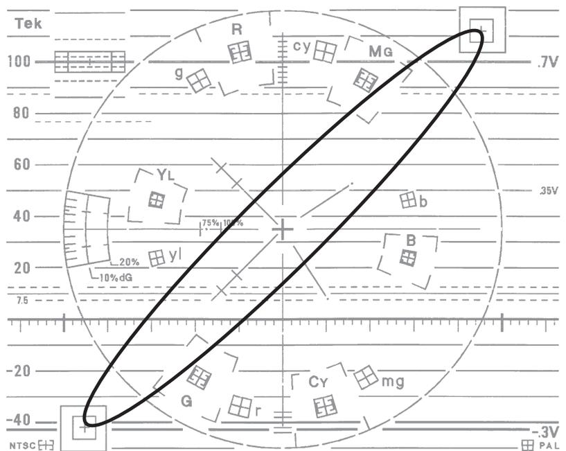
Figure 2-16. Audio display with phase error.
