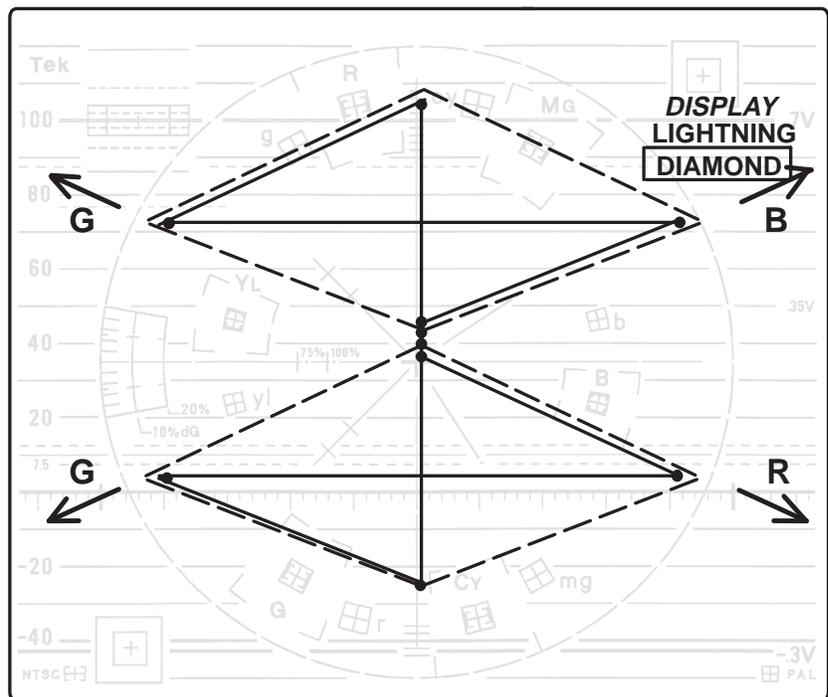
**Figure 4-16.** Diamond display showing signal inside gamut limits.
