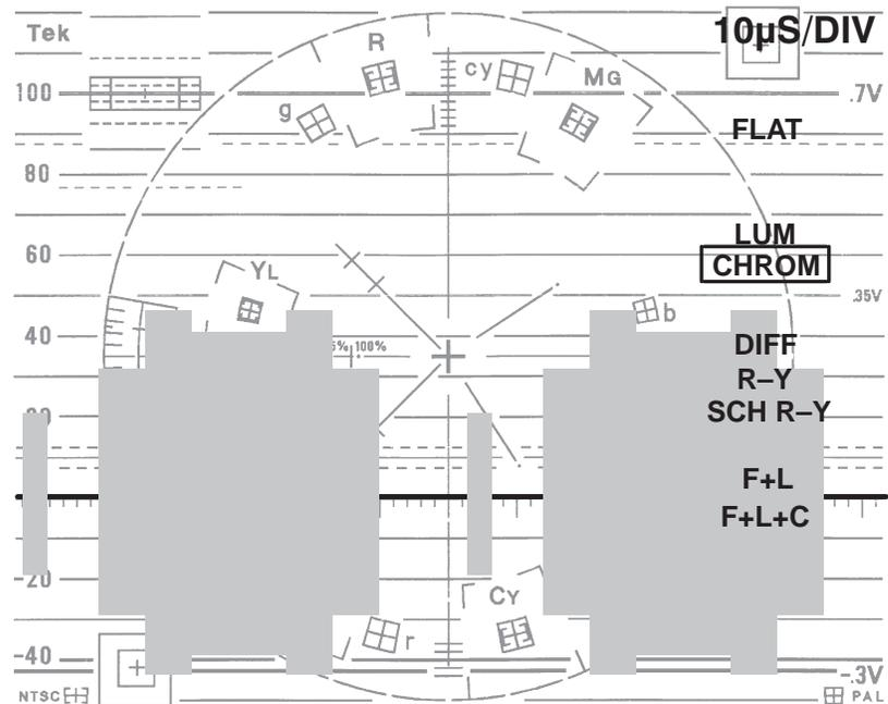
**Figure 2-8.** Two-Line CHROM filter display of color bar signal.
