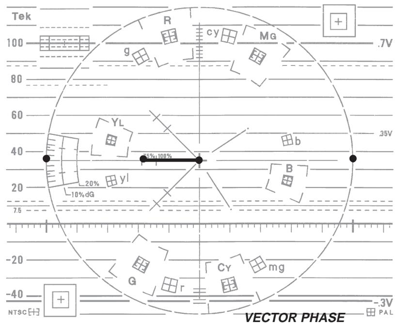
Figure 2-17. NTSC SCH display with internal reference selected.
