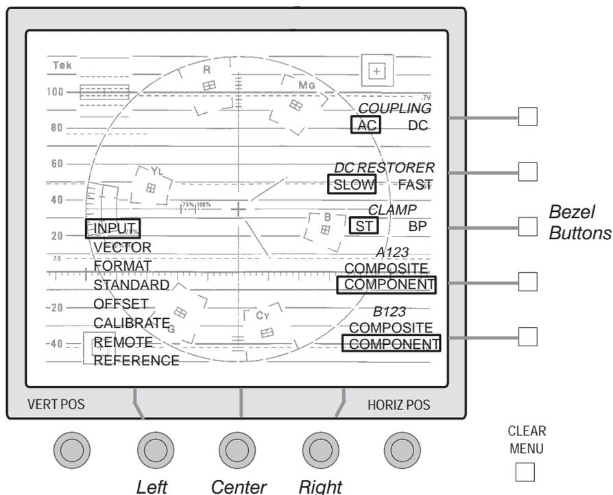
**Figure 3-6.** The CONFIGURE menu display with INPUT selected.
