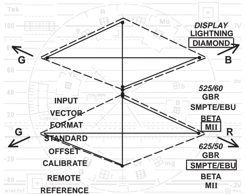
Figure 2-20. Diamond display, showing signal within gamut limit.
