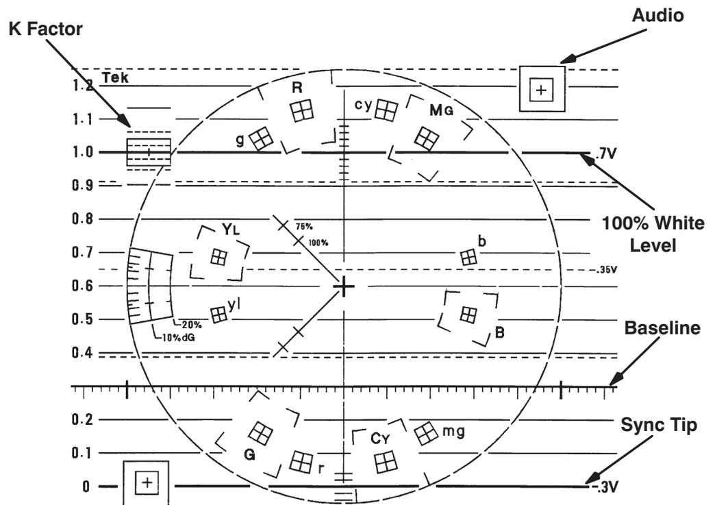
Figure 4-2. PAL waveform/vector graticule.
