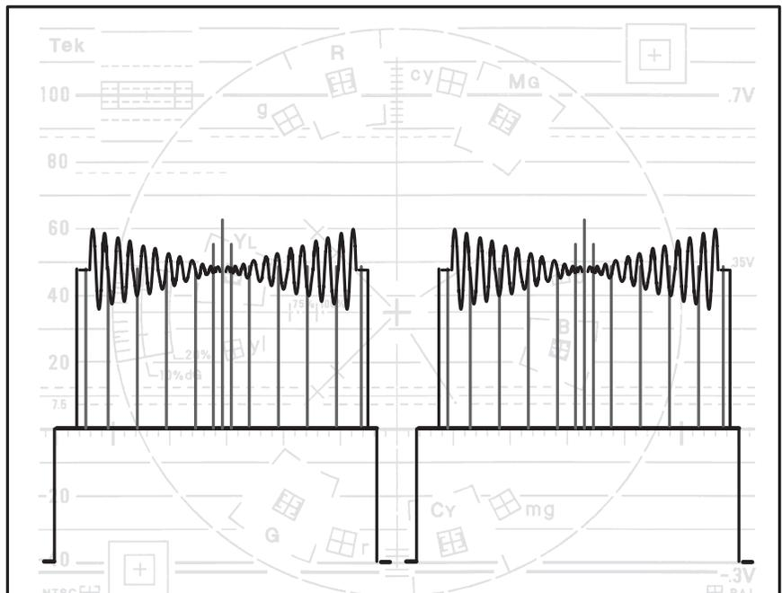
**Figure 4-17.** Bowtie display showing a sharp null.
