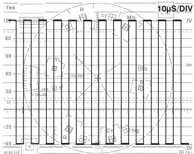
Figure 2-6. Calibrator display.
