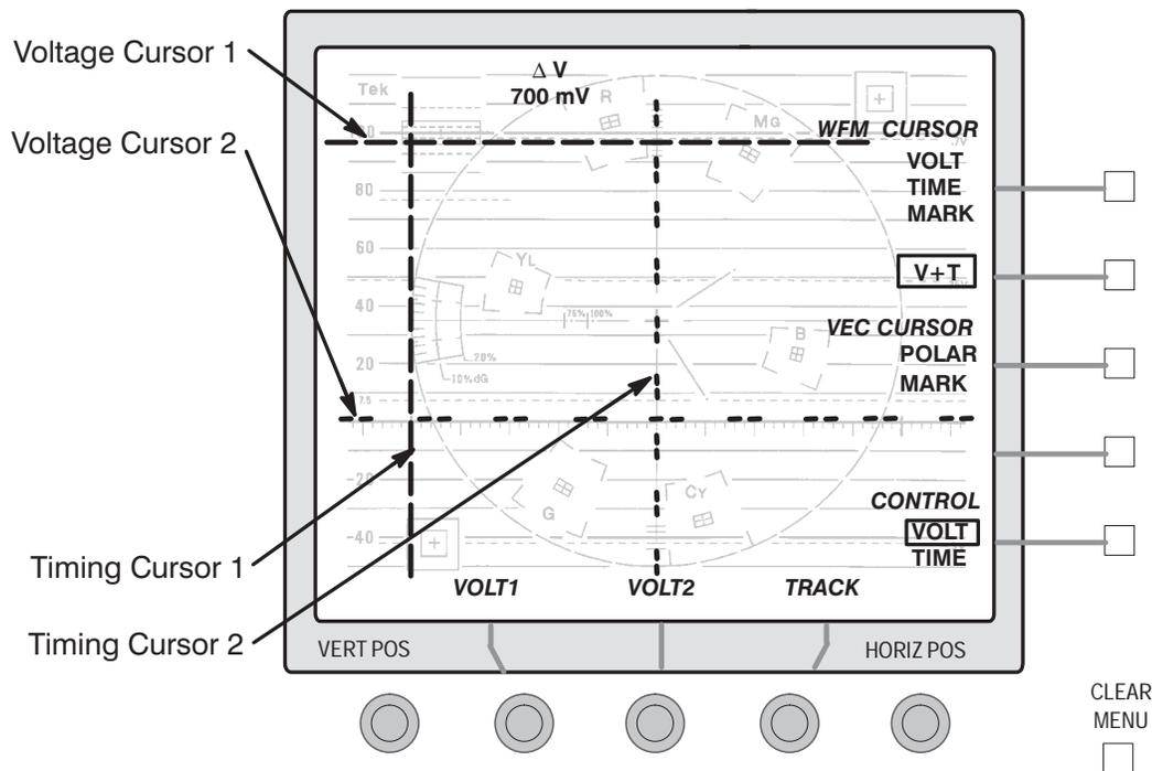
Figure 3-4. The VECTOR+WFM CURSOR menu with V+T selected.
