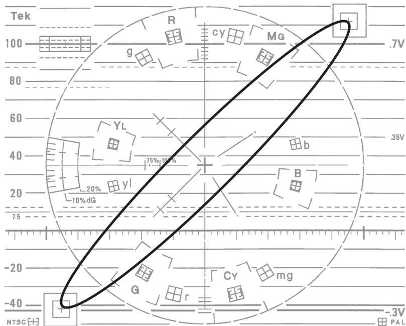
Figure 2-16. Audio display with phase error.
