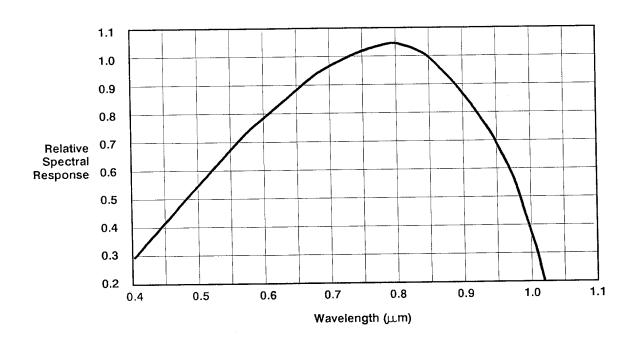
Figure 1-1: Normalized Spectral Response for the P6701A and P6711
