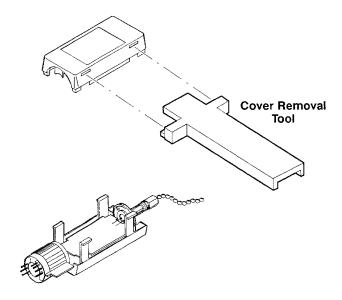
Figure 6-1: Top Cover Removal
