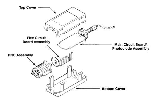
Figure 6-2: Assembly Replacement
