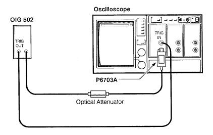
Figure 4-2: Bandwidth Check Setup
