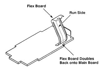
Figure 6-3: Flex Circuit Board Replacement
