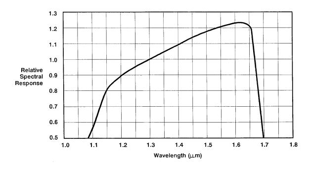
Figure 1-2: Normalized Spectral Response for the P6703A and P6713
