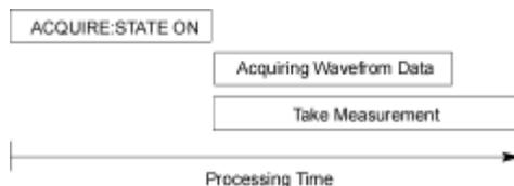
To ensure the instrument completes waveform acquisition before taking the measurement on the acquired data, you can synchronize the program.
