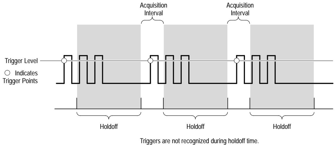
**Figure 3–37: Trigger Holdoff Time Ensures Valid Triggering**
