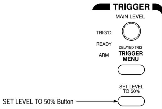
**Figure 2-4: Trigger Controls**
