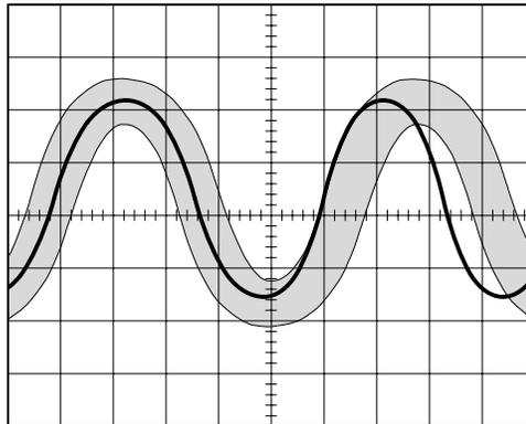
**Figure 3-92: Comparing a Waveform to a Limit Template**
