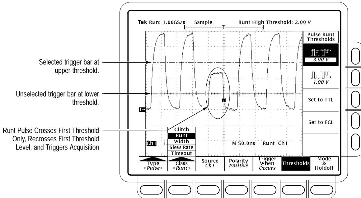
Figure 3-51: Main Trigger Menu — Runt Class
