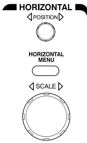
Figure 3–8: Horizontal Controls
