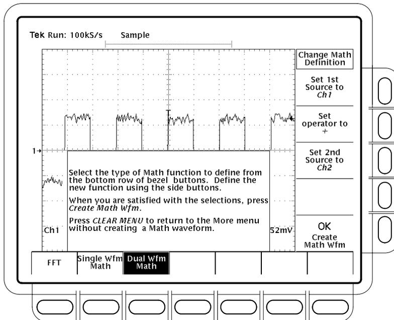
Figure 3–95: Dual Waveform Math Main and Side Menus
