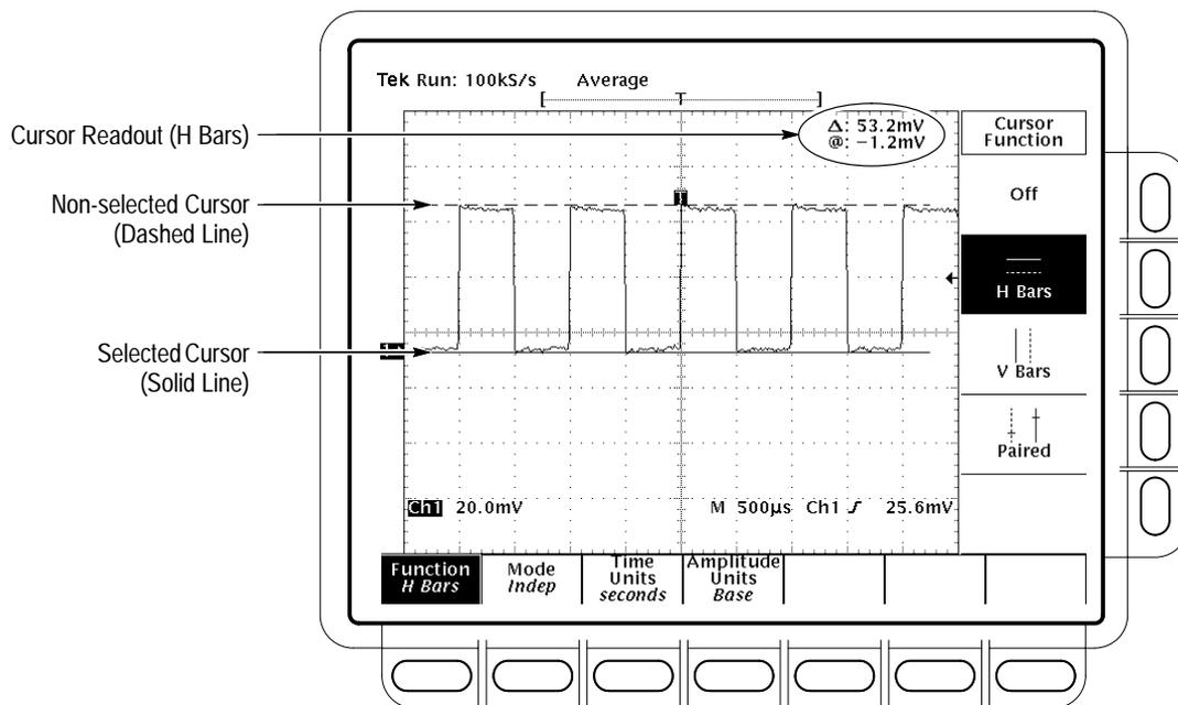
Figure 3–67: H Bars Cursor Menu and Readouts
