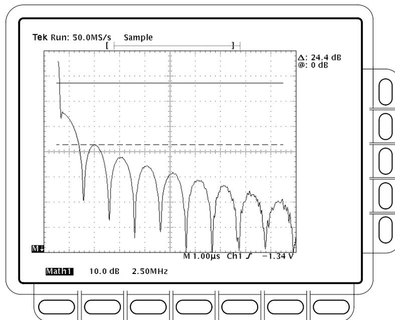
Figure 3–99: Cursor Measurement of an FFT Waveform
