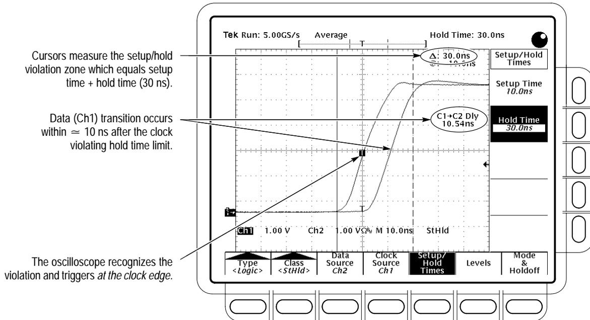
Figure 3–48: Triggering on a Setup/Hold Time Violation
