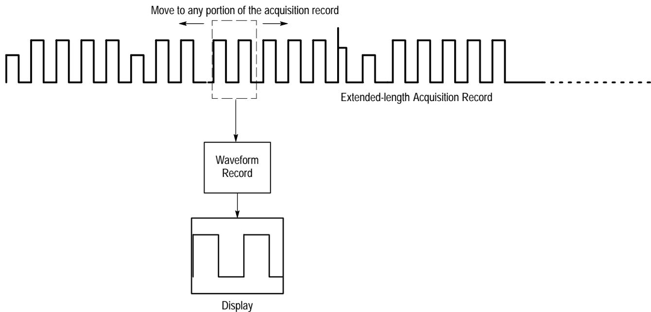
**Figure 3–9: Displaying an Extended Acquisition Length Record**
