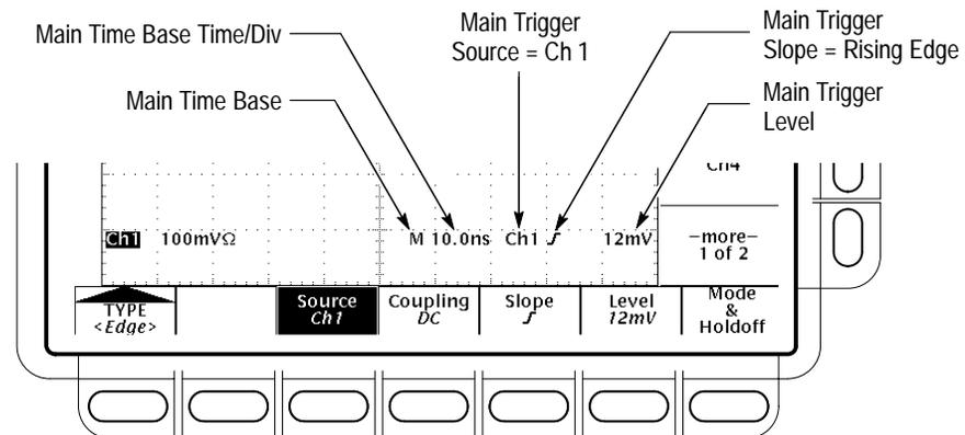
**Figure 3–40: Example Trigger Readouts — Edge Trigger Selected**
