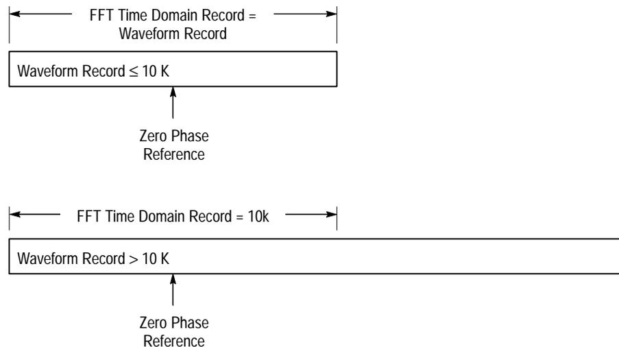
**Figure 3–100: Waveform Record vs. FFT Time Domain Record**
