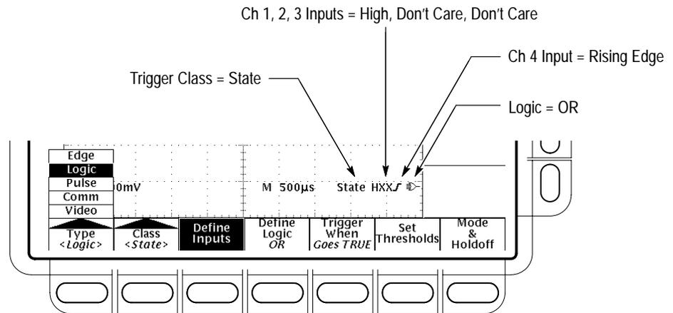
Figure 3-45: Logic Trigger Readouts — State Class Selected
