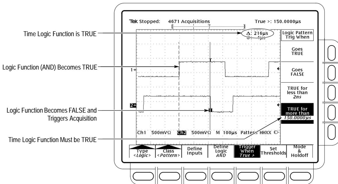
Figure 3–47: Logic Trigger Menu — Time Qualified TRUE
