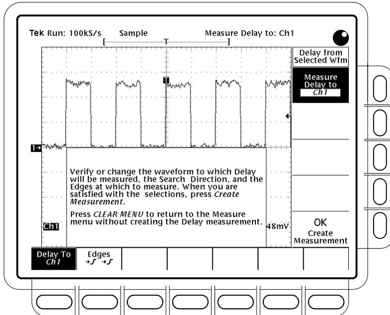
**Figure 3–63: Measure Delay Menu — Delay To**
