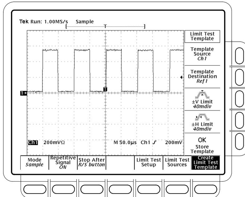
Figure 3-93: Acquire Menu — Create Limit Test Template
