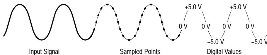
Figure 3–11: Acquisition: Input Analog Signal, Sample, and Digitize
