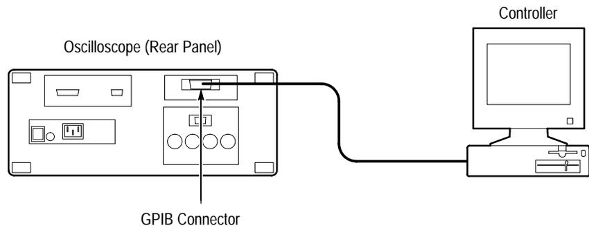
Figure 3–87: Connecting the Oscilloscope to a Controller
