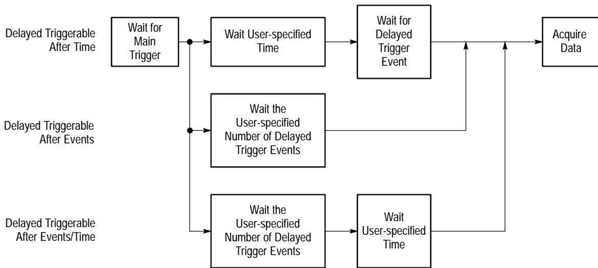
**Figure 3–55: Delayed Triggerable**
