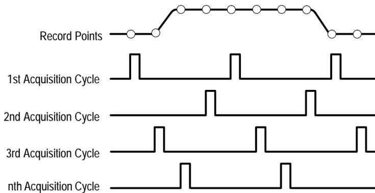
**Figure 3–14: Equivalent-Time Sampling**
