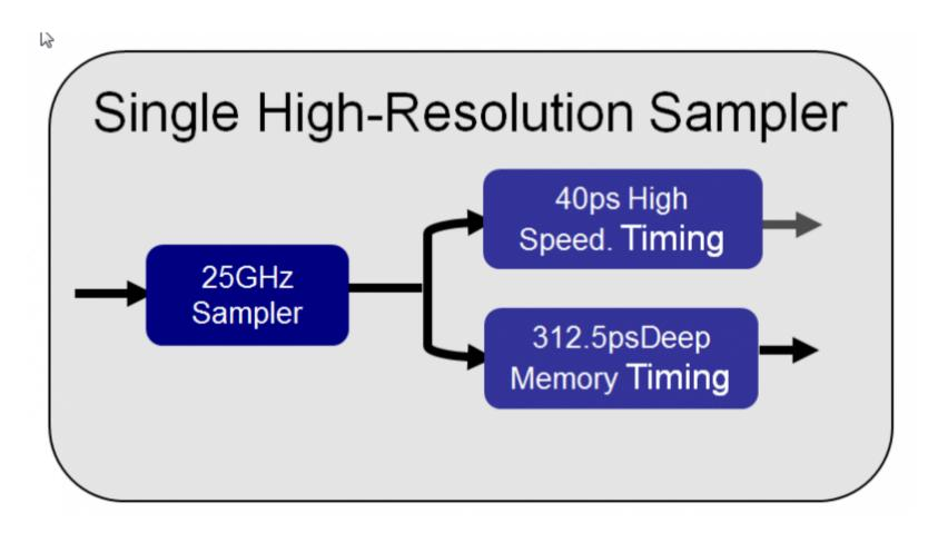
Another powerful feature on a logic analyzer is the suite of tools for analyzing signal integrity issues. For instance, in asynchronous mode, a poor termination or reflection can cause two crossings of a threshold between sample points. This condition is known as a glitch, and some logic analyzers like the TLA6400 can not only trigger on it, but mark the spot in memory where it occurred. In synchronous mode, the logic analyzer can monitor, trigger,
