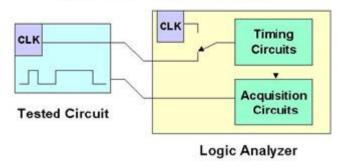
Some more advanced logic analyzers also permit time stamps to be put on the data as it is collected similar to asynchronous mode, but the data itself is only collected and stored on the clock.
