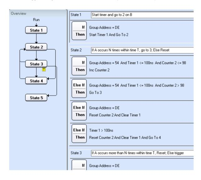
Logic analyzers also have the ability to perform a task called Transitional or Conditional Storage. In this mode, the logic analyzer doesn't store data if the
