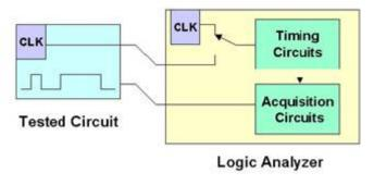
However, the real power of a logic analyzer is in its ability to clock the inputs synchronous to the data being measured, by using an explicitly measured external clock line on the device under test. This mode on a true logic analyzer is called state, synchronous, or external mode. While some MSO's (like
