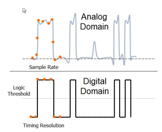
Unlike an MSO or a USB based logic analyzer, a logic analyzer can have over 100 inputs. It also has deeper memory. Many USB based products have less than 100k of memory, whereas a logic analyzer can have over 50 MB of memory. Also, a true logic analyzer typically can acquire at a faster rate. Most USB-based logic analyzers or MSO products go to 1 GS/s, but a logic analyzer like the Tektronix TLA6400 can provide timing resolution to 3.2 GS/s, and high-speed timing to 25 GS/s.
