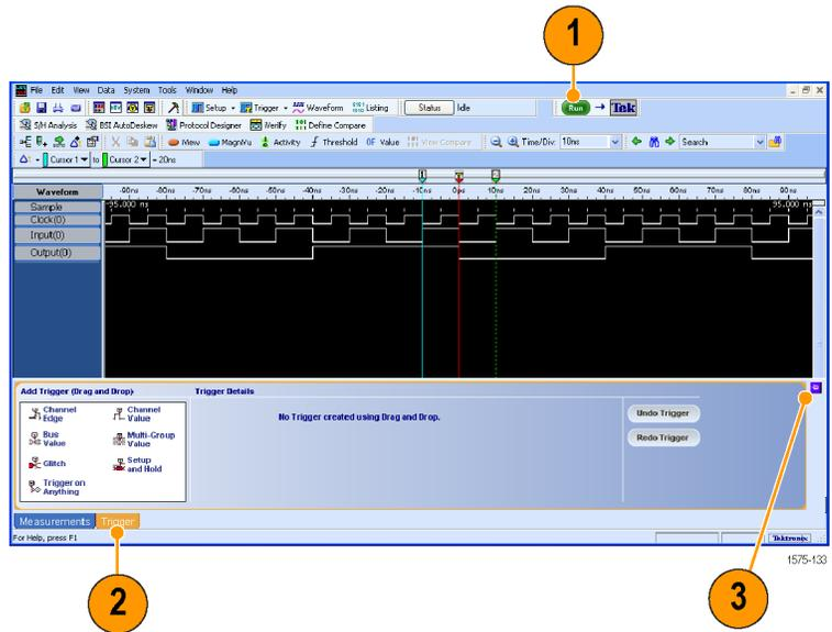
4. Click and drag the **Channel Edge** icon from the Tabbed Trigger window to the Output waveform.
