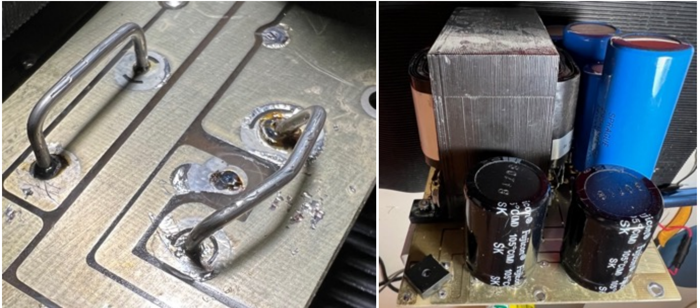
Left: bridges to restore traces continuity. Right: the old (blue) and new (black) capacitors.
