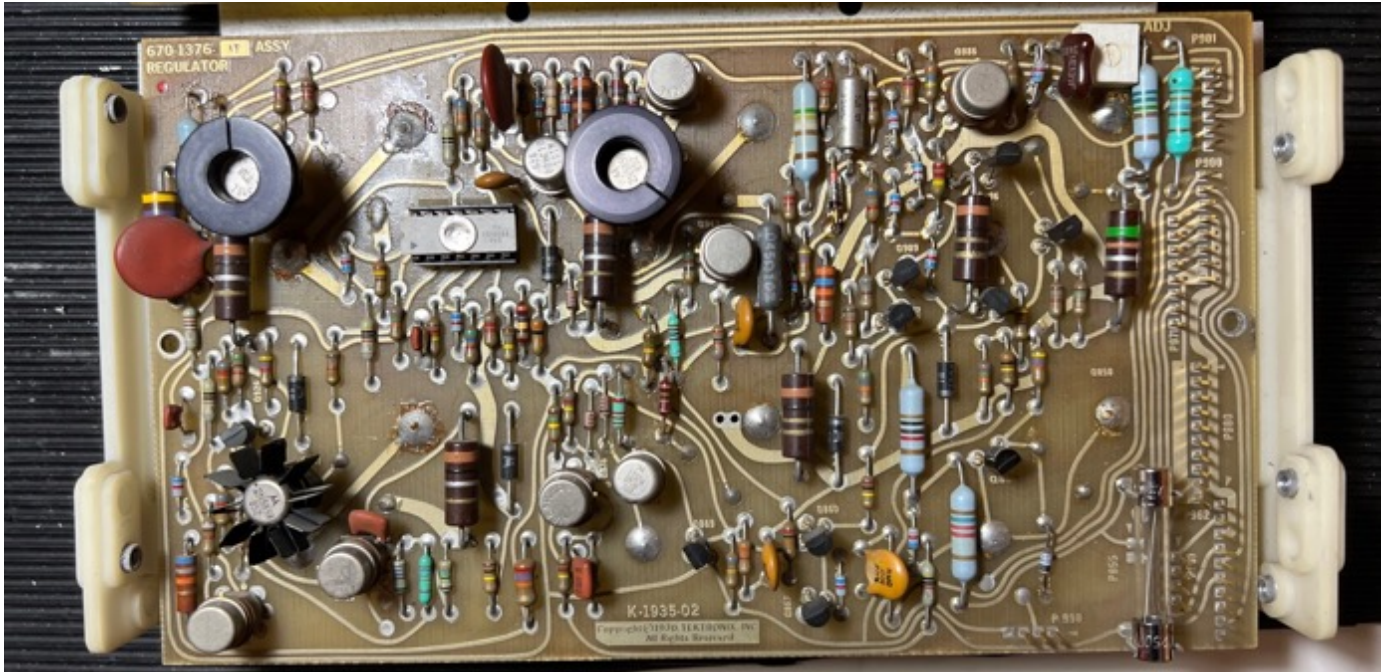
The A11 low voltage (LV) regulator board
