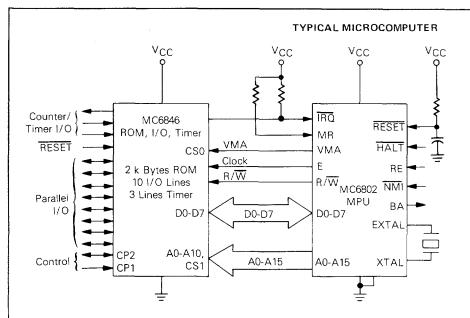
This block diagram shows a typical cost effective microcomputer. The MPU is the center of the microcomputer system and is shown in a minimum system interfacing with a ROM combination chip. It is not intended that this system be limited to this function but that it be expandable with other parts in the M6800 Microcomputer family.
