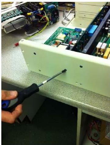
**REMOVE SIDE FIXING SCREWS WHICH HOLD
