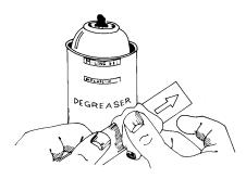
Thoroughly degrease the gaging area with solvent, such as CSM Degreaser or GC-6 Isopropyl Alcohol. The former is preferred, but there are some materials (e.g., titanium and many plastics) that react with CSM. In these cases, GC-6 Isopropyl Alcohol should be considered. All degreasing should be done with uncontaminated solvents-thus the use of "one-way" containers, such as aerosol cans, is highly advisable.
