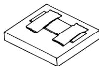
4. Partially remove the gage from its acetate folder so that the top half of the gage (grid end) is exposed.
