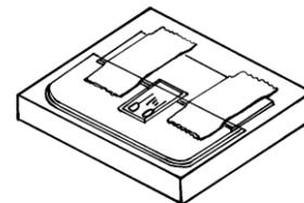
7. While maintaining pressure, fold the carrier back over the folder and peel straight back with a smooth, steady pull. Use only sufficient pressure to allow folder to slide as the carrier is peeled against it. This technique minimizes stretch in the carrier and curling of the gage filament.
