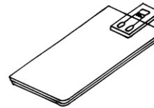
5. With foil side of the gage facing down, position it on the exposed mastic of the tape so that half the length of each endloop contacts the lower edge of the tape. Remove acetate folder, but do not discard. Press down firmly on the gage carrier with stick end of a cotton applicator to anchor the foil to the tape mastic.
