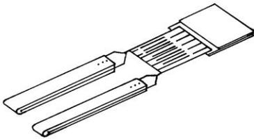
10. Place the gage on a cleaned copper plate and slip the lead over the gage tabs, forming a "sandwich" effect with the tab between the two Nichrome V lead ribbon ends.
