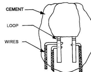
2. Fold the lead ribbons over the top of wires. Place a thin strip of copper under the ribbons.
