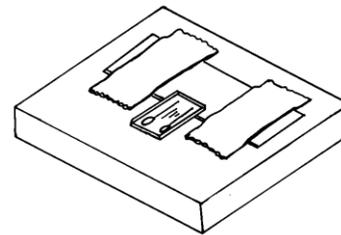
6. Place the acetate folder over the gage carrier, aligning sealed edge with top of gage endloops. Press lightly on the acetate folder and loosen the end of the gage carrier from tape mastic with a pair of tweezers.
