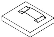
3. Tape the folds of the gage installation tape firmly to the surface with two pieces of drafting tape, leaving the center of the gage installation tape exposed approximately 1.5 times the width of gage carrier.
