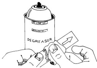
The surface preparation technique used is the same basic cleaning procedure described in Micro-Measurements Instruction Bulletin B-129, "Surface Preparation for Strain Gage Bonding". The initial step is to thoroughly degrease
