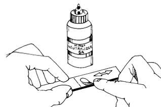
Apply a liberal amount of M-Prep Neutralizer 5A to the gage area. Keeping the surface wet, scrub with cotton tipped applicators. Do not allow evaporation of the cleaning material on the specimen surface since this would leave a thin, unwanted film between the adhesive and the specimen. Remove the Neutralizer by slowly wiping through the gage area, allowing the gauze sponge to absorb the Neutralizer. Do not wipe back and forth over
