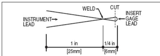
Insert the gage lead between the two 0.25 in [6mm] ends of the transition ribbons, and spot weld at a minimum of three points using the Micro-Measurements Model 700 spot welder and tweezer handpiece. Repeat for the second lead.
