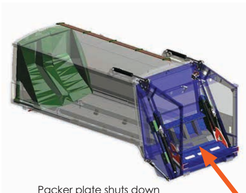
Packer plate shuts down when maximum load is reached
