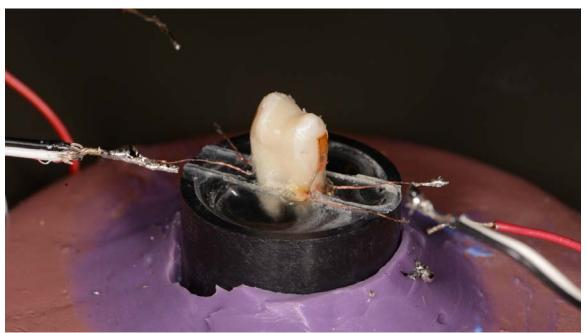
Figure 2: Maxillary premolar mounted in a phenolic ring with Micro-Measurements model EA-06-062AP-120/LE strain gages bonded.
