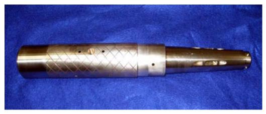
Figure 1: Hybrid force balance
