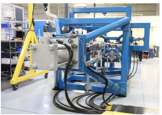
Image 3: Horizontal fatigue test frame
