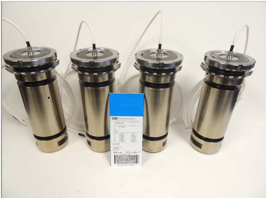
Additionally, Advanced Sensors technology allows for better gage matching, tighter resistance tolerance, and more repeatability through temperature. The modified Karma foil used to manufacture these gages is produced in-house (a Micro-Measurements exclusive) to ensure the greatest uniformity from gage to gage and maximizing output stability.
