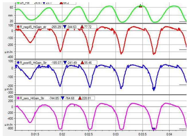
Figure 5: Trailing arm data collected from strain gage rosette and linear potentiometer.
