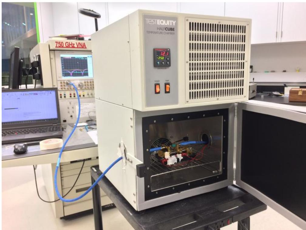
Fig.5 — Outside of the temperature chamber
