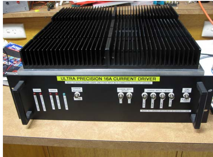
Figure 2: View of the 16 A precision current driver. The massive heatsink removes heat from the shunt resistor, via the Peltier modules, as well as from the linear series-pass regulator MOSFETs.
