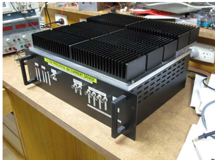
Figure 3: A cooling fan cannot be used, as the rotating stray magnetic field would inject noise into the sensitive circuitry.
