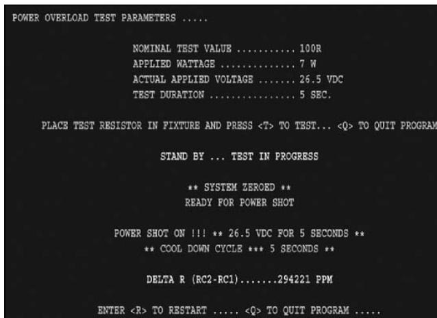
Figure 3. STO for thin film resistor
