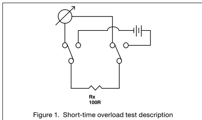
Figure 1. Short-time overload test description
