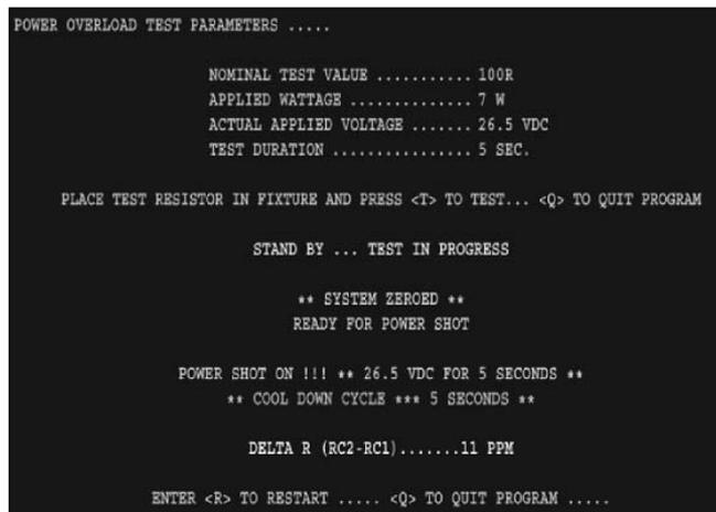
Figure 2. STO for Bulk Metal<sup>®</sup> Foil resistor
