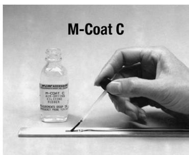
To ensure these problems are not encountered, Micro-Measurements offers three qualified RTV silicone rubber coatings which produce a safer methyl alcohol
