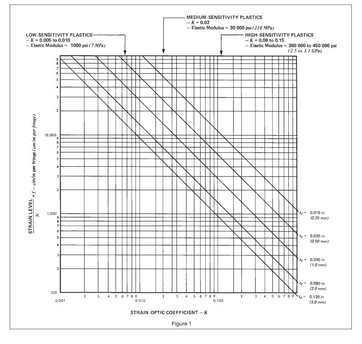
(For use with non-standard coating thicknesses, additional thickness lines between 0.010 in [0.25 mm] and 0.120 in [3 mm] can be plotted on the graph as necessary.) If no such intersection can be found, it will generally be necessary to accept a lower sensitivity and work with fewer fringes. The following exercise will illustrate the procedure.
