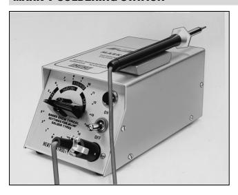
A time-proven precision soldering instrument for miniature and/or delicate soldering applications. Full 25-watt rating in 17 selector positions to handle all *M-LINE* solder alloys listed on page 52. Magnetic solder pencil holder and flexible, burn-resistant cord. Lightweight soldering pencil [1.1oz (31g)]. Operates on 50 or 60Hz. Specify 115 or 230Vac.
