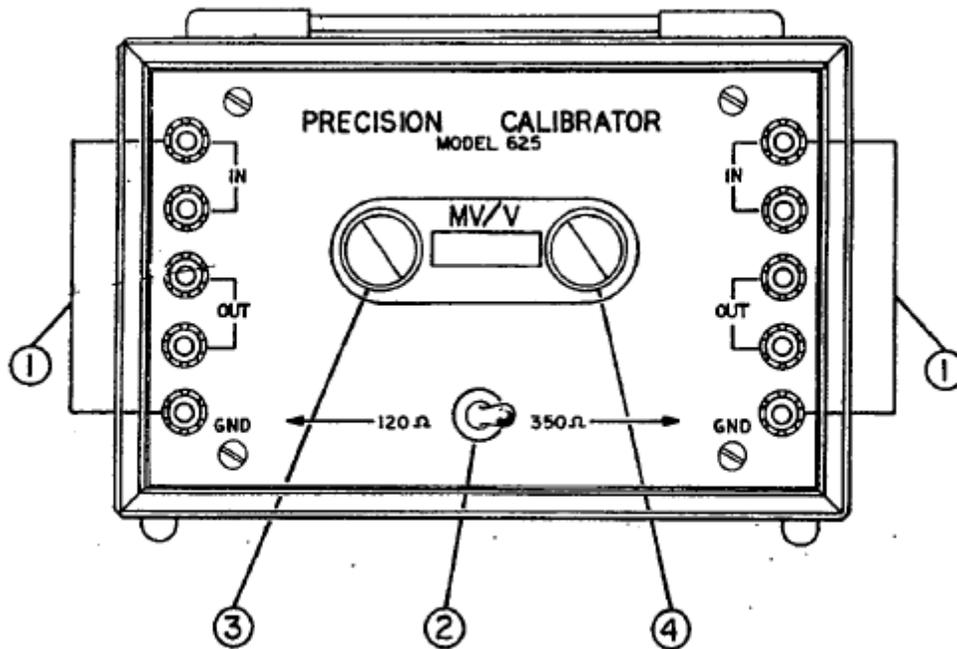
1. Color-coded Binding Posts. Right side posts are used for 350 $\Omega$  connections; left side posts for 120 $\Omega$  connections.
