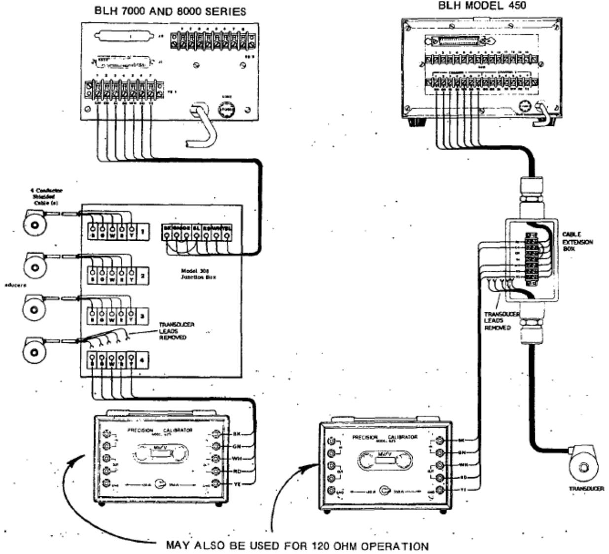
Figure 2-3. 625 Connections to J-Box and Extension Box
