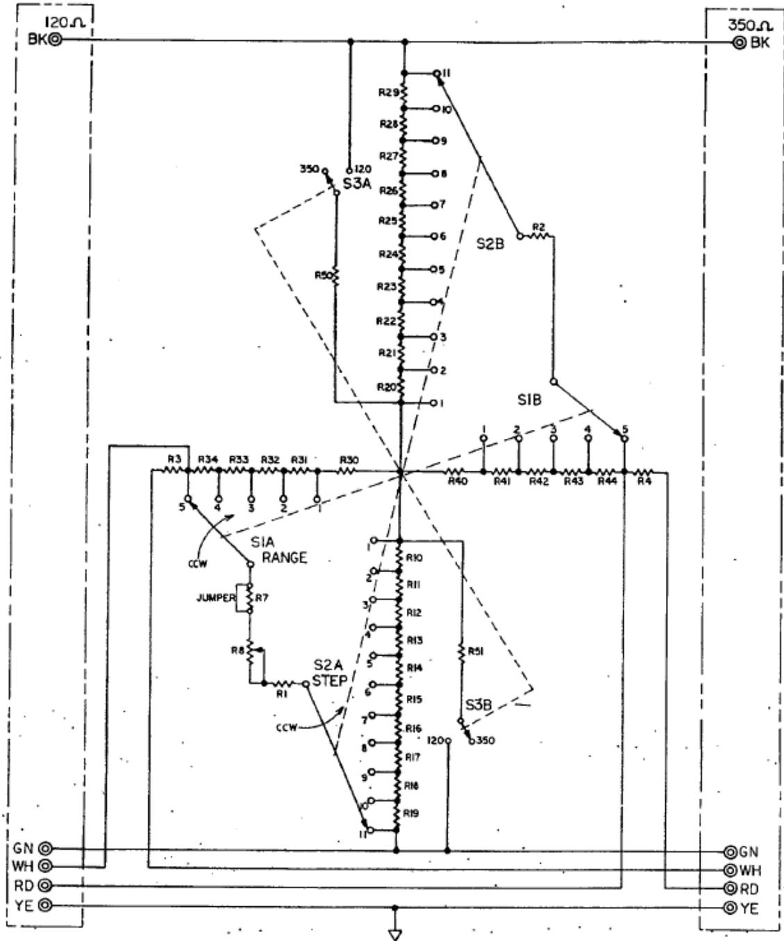
Figure 4-1. Model 625 Schematic Diagram
