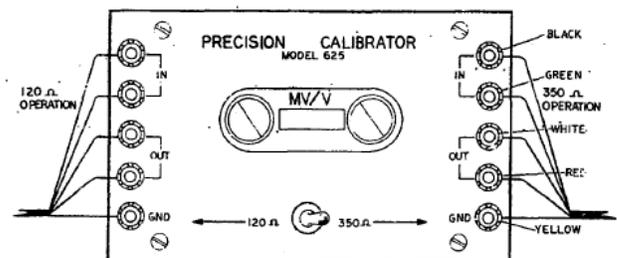
Figure 2-1. Model 625 Connections.
