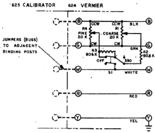
Figure 4-2. Model 624 Schematic Diagram
