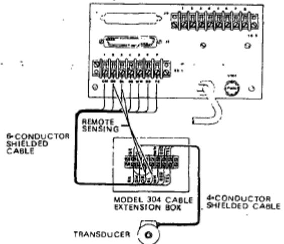
Figure 2-5, Remote Sensing Connections.
