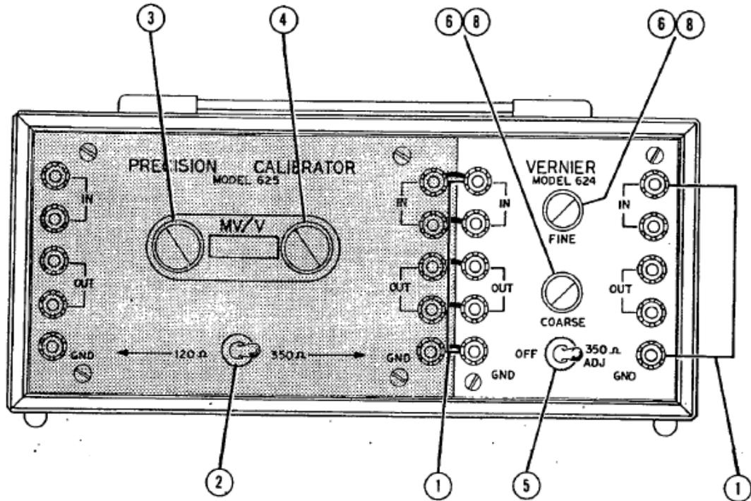
1. Attach the 5-conductor cable to the right-side binding posts ( paragraph 2-34 ). Left-side binding posts MUST be bussed to the Model 625.
