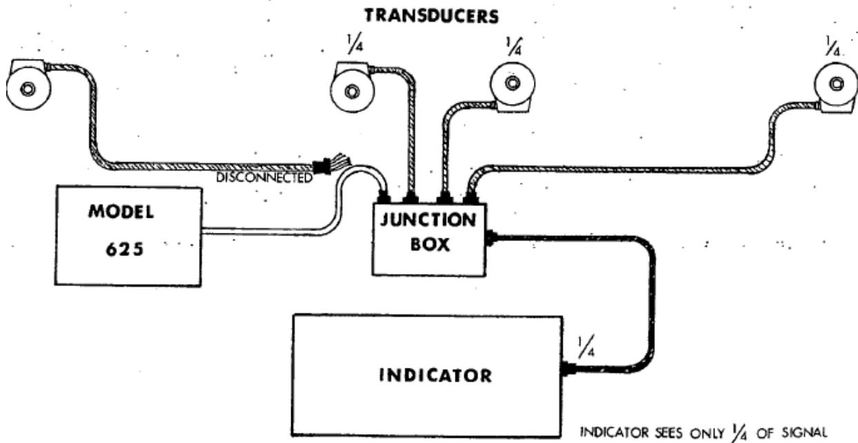
**Figure 3-2. Four Transducer System Calibration.**
