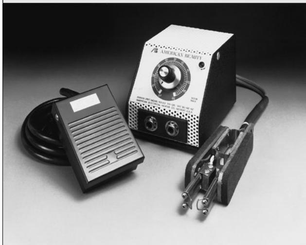
The ease and simplicity of operation of the Thermal Wire Stripper make it ideal for most strain gage leadwire stripping. The variable heat control allows stripping of all thermoplastic insulations, including Teflon®, in sizes No. 18 to No. 36 AWG (1 to 0.1 mm diameter). The foot switch and tweezers hand-piece give excellent operator control over the stripping operation. Includes power unit and foot switch, both with 3-wire NEMA plugs, and tweezers handpiece.
