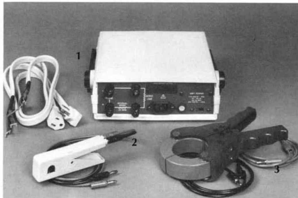
Rear view of a Valhalla 2100 Series Wattmeter with accessories. Item 1 is the option "X21" load extension cord. Item 2 is the option "I-150" 150 Amp clamp-on C.T. item 3 is the option "I-1000" 1000 Amp Transformer.
