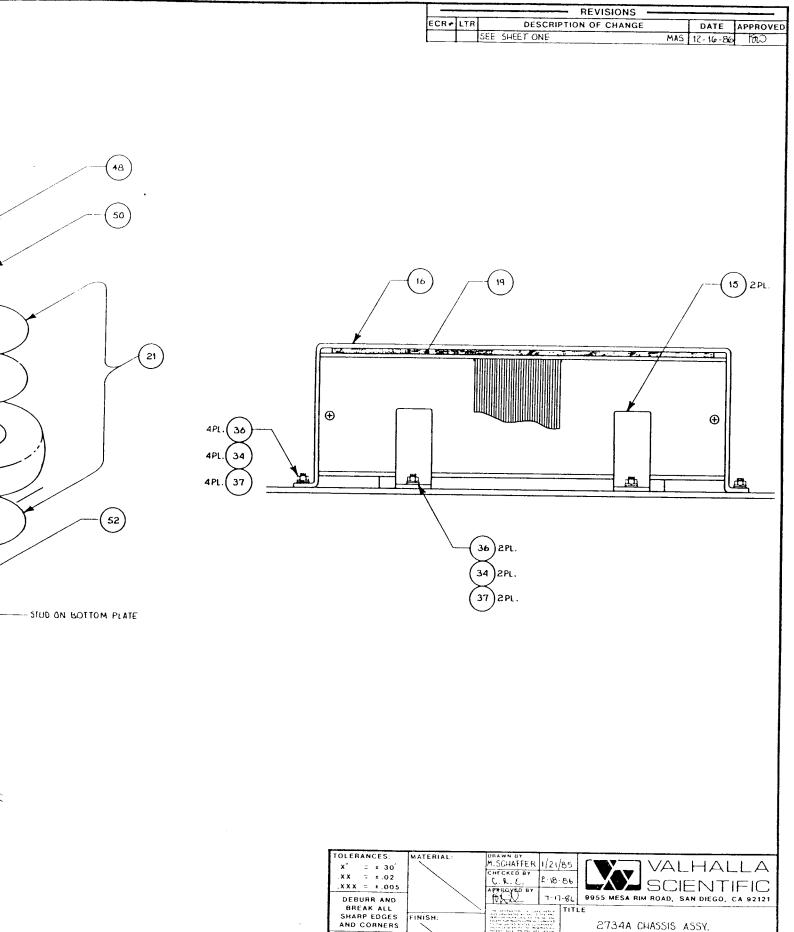
BREAK ALL SHARP EDGES AND CORNERS MACHINED SURFACES ARE TO HAVE A FINISH OF 63/ SHEET 2 OF 5 NONE BREAK ALL 2734A CHASSIS ASSY. BREAK NO. 2734-400 B
