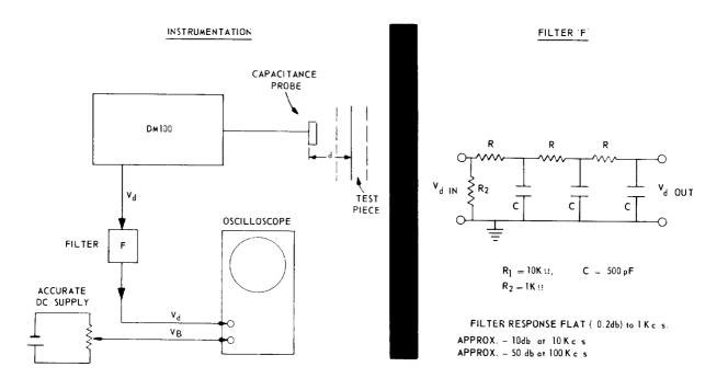
When the test specimen is vibrated, the spot will follow the excursion of the specimen; a typical sensitivity would be 4 micro-inches vibration amplitude (peak to peak) for 1 cm oscilloscope deflection on an oscilloscope range of 4 mv/cm range.
