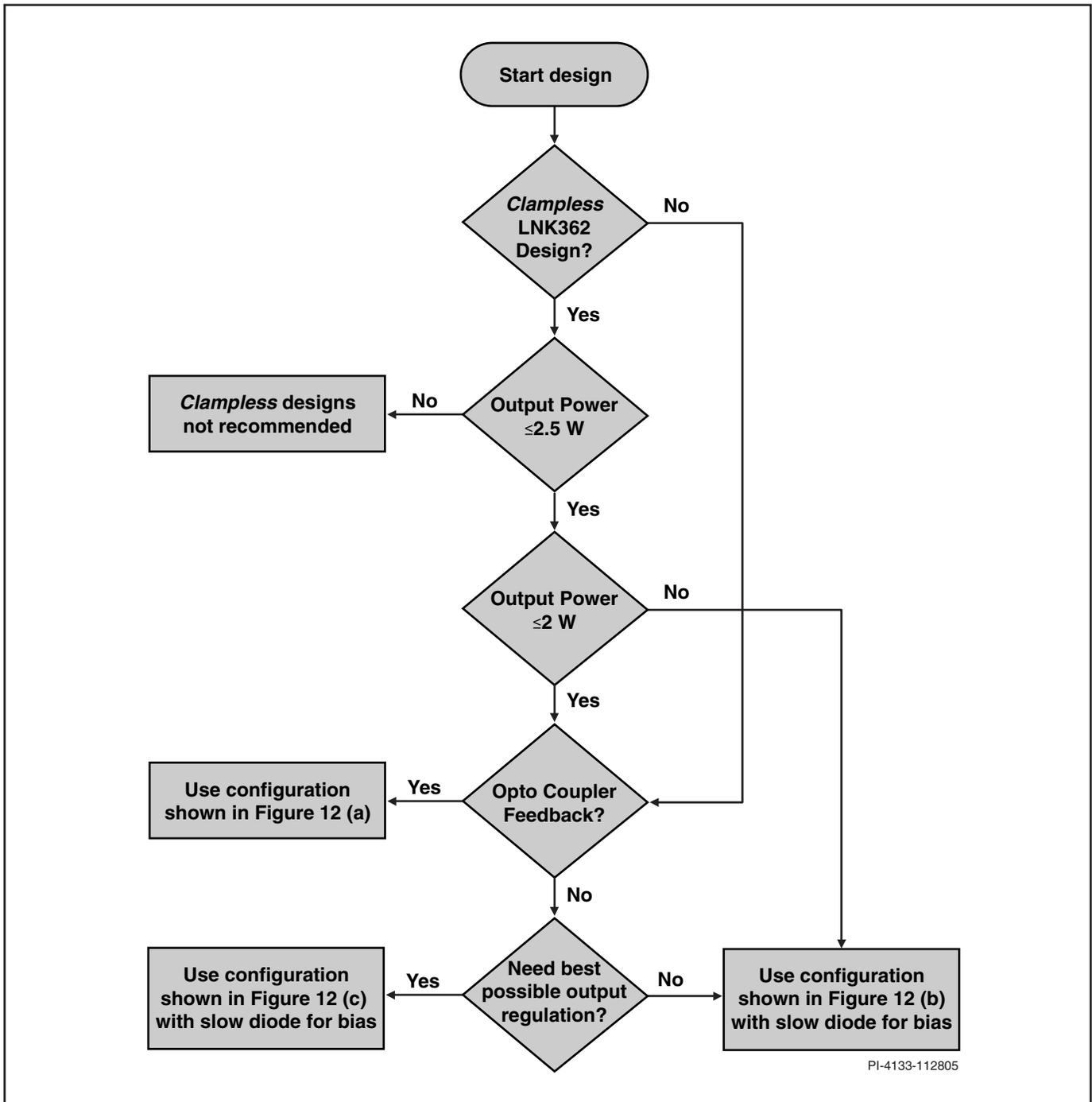
Figure 11. Flowchart For Deciding Mechanical Structure of Transformer.
