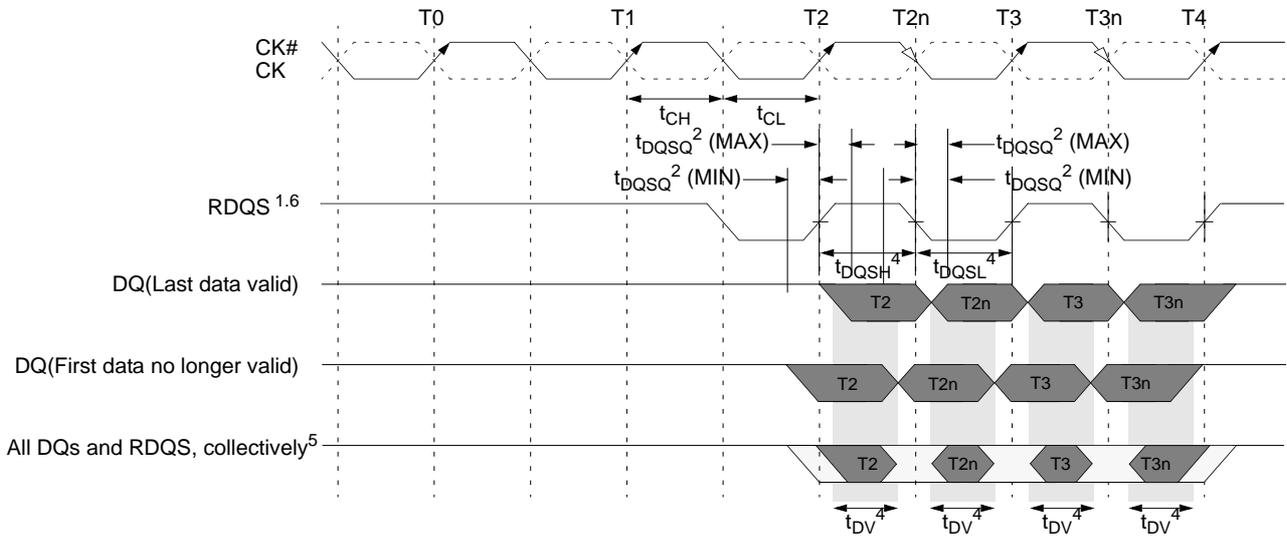
Data Output Timing (2) -  $t_{DQSQ}$ ,  $t_{QH}$  and Data Valid Window
