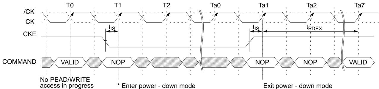
\* Once the device enters the power down mode, it should be in NOP state at least for 10ns
