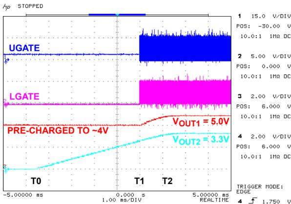
FIGURE 6. ISL6549EVAL1 START-UP INTO A PARTIALLY CHARGED OUTPUT
