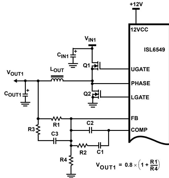
FIGURE 20. ADJUSTING  $V_{OUT1}$
