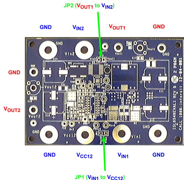
FIGURE 1. ISL6549EVAL1 INPUT AND OUTPUT CONNECTIONS
