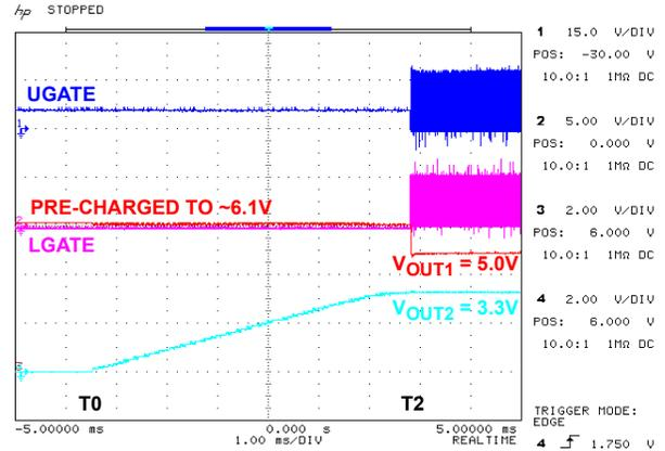
FIGURE 7. ISL6549EVAL1 START-UP INTO AN OVER-CHARGED OUTPUT
