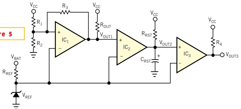
The additional comparator in Figure 5 switches when the exponential signal reaches  $V_{REF}$ .
