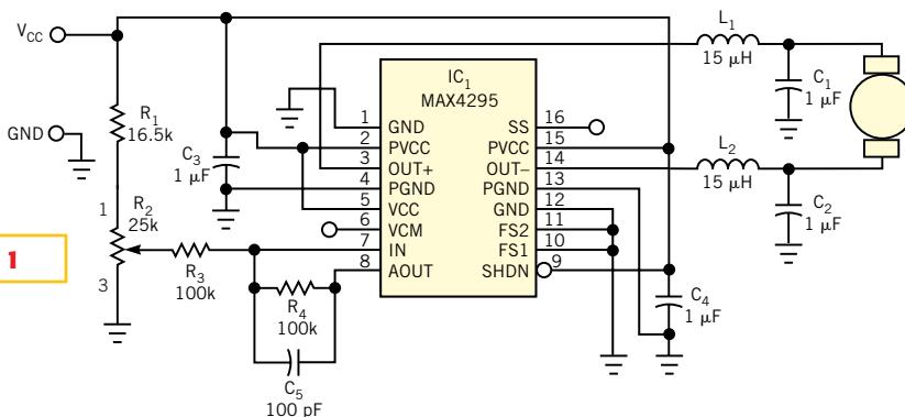
**A Class D audio amplifier, IC<sub>1</sub>, helps implement this simple motor-speed controller.**
