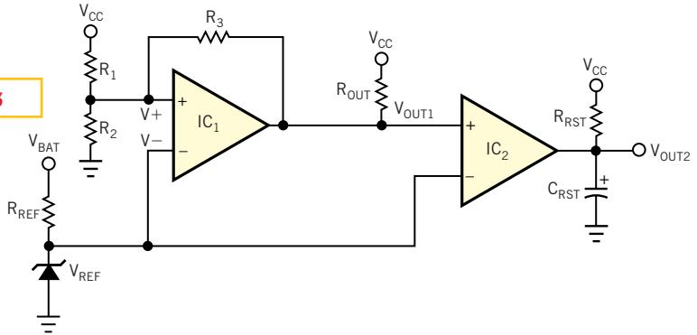
This circuit introduces a time constant in the reset function.
