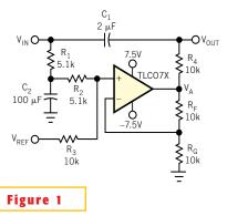
This circuit is a universal level shifter for ac signals; it accommodates any interface standard.
