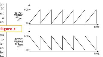
The up ramp of the upper waveforms occurs at the same time as the down ramp of the bottom waveform.
