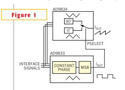
Two DDS chips provide a convenient way to generate sawtooth waveforms.
