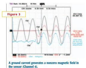
rent difference is null. **Figure 3** shows a ground current that generates a nonzero magnetic field in the sensor. In **Figure 4**, the ground current is greater than 30 mA. The comparator changes state, activating the optotriac (Channel 1)
