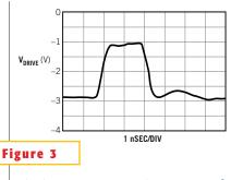
The driver in Figure 1 switches 1.6V into  $75\Omega$  with less-than-1-nsec rise and fall times.
