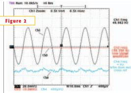
The sensor's output (Channel 4) is zero because the differential line current is zero.
