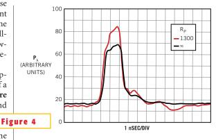
These curves show the VCSEL's response with  $R_p$  open and  $R_p$ =1300 $\Omega$ .
