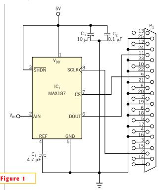
It's easy to effect an interface of a 12-bit serial ADC to a PC.
