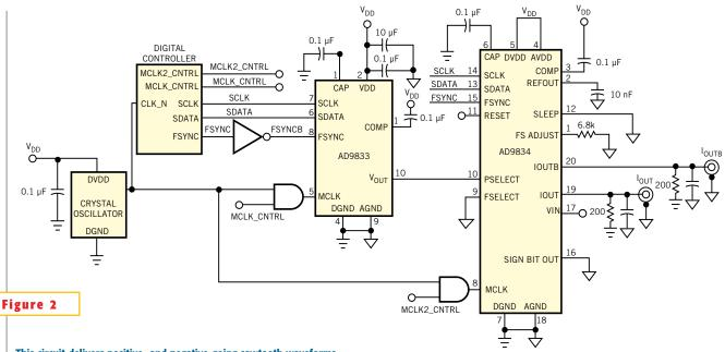
This circuit delivers positive- and negative-going sawtooth waveforms.
