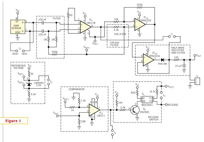
This circuit uses a GMR sensor to detect and disable dangerous differential line currents.
