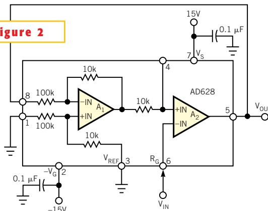
**This companion circuit to the one in Figure 1 delivers an accurate gain of  $-10$ .**
