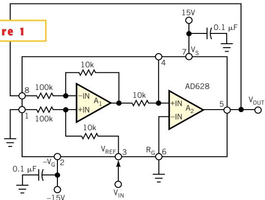
**This circuit has a precise gain of 10 and uses no external components.**
